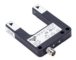
AutomationDirect photoelectric fork sensor, U-frame, die-cast zinc housing, through-beam, infrared, 0-30mm sensing distance, 10-30 VDC operating voltage, selectable light-on/dark-on, NPN, 3-pin M8 quick-disconnect.
