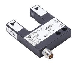
AutomationDirect photoelectric fork sensor, U-frame, die-cast zinc housing, through-beam, infrared, 0-20mm sensing distance, 10-30 VDC operating voltage, selectable light-on/dark-on, NPN, 3-pin M8 quick-disconnect.
