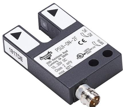
AutomationDirect photoelectric fork sensor, U-frame, die-cast zinc housing, through-beam, infrared, 0-10mm sensing distance, 10-30 VDC operating voltage, selectable light-on/dark-on, NPN, 3-pin M8 quick-disconnect.
