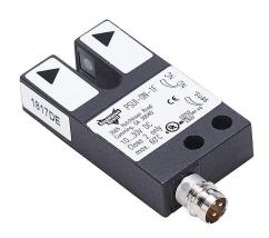
AutomationDirect photoelectric fork sensor, U-frame, die-cast zinc housing, through-beam, infrared light emission, 0-5mm sensing distance, 10-30 VDC operating voltage, selectable light-on/dark-on, NPN, 3-pin M8 quick-disconnect.
