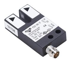
AutomationDirect photoelectric fork sensor, U-frame, die-cast zinc housing, through-beam, infrared, 0-5mm sensing distance, 10-30 VDC operating voltage, selectable light-on/dark-on, NPN, 3-pin M8 quick-disconnect.
