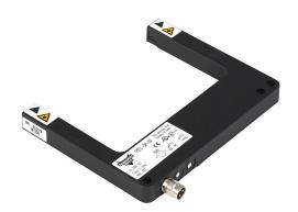
AutomationDirect photoelectric fork sensor, U-frame, die-cast zinc housing, through-beam, clear object detection, Class 1 laser light emission, 0-80mm sensing distance, 10-30 VDC operating voltage, selectable light-on/dark-on, PNP, 3-pin M8 quick-disconnect.
