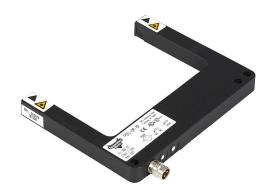
AutomationDirect photoelectric fork sensor, U-frame, die-cast zinc housing, through-beam, clear object detection, Class 1 red laser, 0-80mm sensing distance, 10-30 VDC operating voltage, selectable light-on/dark-on, PNP, 3-pin M8 quick-disconnect.
