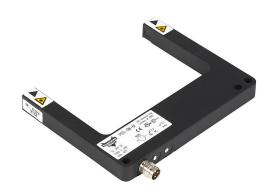
Photoelectric fork sensor, through-beam, clear object detection,  $100 \times 88 \times 10$ mm, U-frame, Class 1 laser light emission, 0-80mm sensing distance, 10-30 VDC operating voltage, NPN, IP67, 3-pin M8 quick-disconnect.
