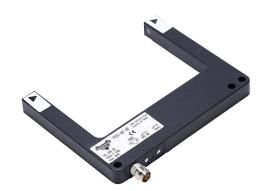
AutomationDirect photoelectric fork sensor, U-frame, die-cast zinc housing, through-beam, liquid detection, infrared light emission, 0-80mm sensing distance, 10-30 VDC operating voltage, selectable light-on/dark-on, PNP, 3-pin M8 quick-disconnect.
