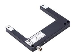
AutomationDirect photoelectric fork sensor, U-frame, die-cast zinc housing, through-beam, liquid detection, infrared, 0-80mm sensing distance, 10-30 VDC operating voltage, selectable light-on/dark-on, PNP, 3-pin M8 quick-disconnect.
