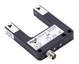
AutomationDirect photoelectric fork sensor, U-frame, die-cast zinc housing, through-beam, liquid detection, infrared, 0-30mm sensing distance, 10-30 VDC operating voltage, selectable light-on/dark-on, PNP, 3-pin M8 quick-disconnect.
