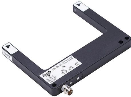
AutomationDirect photoelectric fork sensor, U-frame, die-cast zinc housing, through-beam, liquid detection, infrared, 0-80mm sensing distance, 10-30 VDC operating voltage, selectable light-on/dark-on, NPN, 3-pin M8 quick-disconnect.
