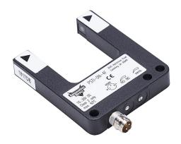
AutomationDirect photoelectric fork sensor, U-frame, die-cast zinc housing, through-beam, liquid detection, infrared, 0-30mm sensing distance, 10-30 VDC operating voltage, selectable light-on/dark-on, NPN, 3-pin M8 quick-disconnect.
