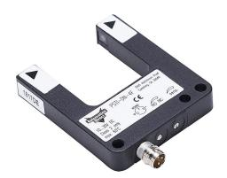
AutomationDirect photoelectric fork sensor, U-frame, die-cast zinc housing, through-beam, liquid detection, infrared light emission, 0-30mm sensing distance, 10-30 VDC operating voltage, selectable light-on/dark-on, NPN, 3-pin M8 quick-disconnect.
