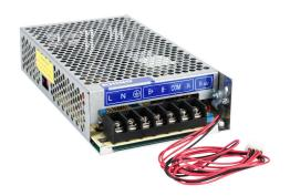
RHINO SELECT PSS series switching power supply, 27.8 VDC @ 5.5A/151W (adjustable), 120/240 VAC nominal input, 1-phase, enclosed, galvanized steel housing, chassis mount, screw terminals.
