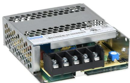
RHINO PSS series switching power supply, 24 VDC @ 1.5A/35W (adjustable), 100-240 VAC nominal input, 1-phase, enclosed, aluminum housing, chassis mount, screw terminals.
