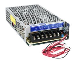
RHINO SELECT PSS series switching power supply, 13.8 VDC @ 11A/151W (adjustable), 120/240 VAC nominal input, 1-phase, enclosed, galvanized steel housing, chassis mount, screw terminals.
