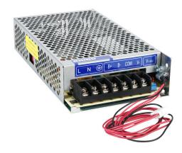
RHINO SELECT PSS series switching power supply, 13.8 VDC @ 11A/151W (adjustable), 120/240 VAC nominal input, 1-phase, enclosed, galvanized steel housing, chassis mount, screw terminals.
