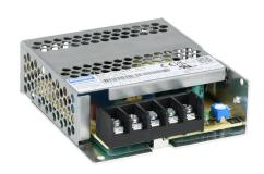
RHINO PSS series switching power supply, 12 VDC @ 4.2A/50W (adjustable), 100-240 VAC nominal input, 1-phase, enclosed, aluminum housing, chassis mount, screw terminals.
