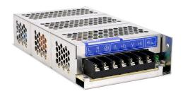
RHINO PSS series switching power supply, 24 VDC @ 2.7A/100W (adjustable) and 5 VDC @ 0.5A/35W, 120/240 VAC or 125-375 VDC nominal input, 1-phase, enclosed, aluminum housing, chassis mount, screw terminals.
