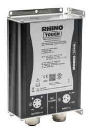
RHINO TOUGH PSRT series switching power supply, 24 VDC @ 8A/192W, 120/240 VAC nominal input, 1-phase, encapsulated, aluminum housing, chassis mount, (1) 7/8in - 16 UN2 3-pin male and (1) 7/8in - 16 UN2 5-pin female.
