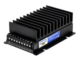
RHINO PRO DC to DC converter, 9-36 VDC input, 48 VDC output, 3.2A, 150W, aluminum housing, encapsulated, chassis mount, screw terminal.
