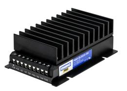
RHINO PRO DC to DC converter, 9-36 VDC input, 28 VDC output, 5.4A, 150W, aluminum housing, encapsulated, chassis mount, screw terminal.
