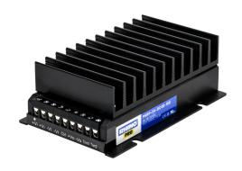
RHINO PRO DC to DC converter, 18-75 VDC input, 24 VDC output, 6.3A, 150W, aluminum housing, encapsulated, chassis mount, screw terminal.
