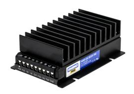
RHINO PRO DC to DC converter, 9-36 VDC input, 24 VDC output, 6.3A, 150W, aluminum housing, encapsulated, chassis mount, screw terminal.
