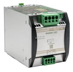
RHINO PRO PSRP series switching power supply, 24 VDC @ 40A/960W (adjustable), 480 VAC nominal input, 3-phase, enclosed, aluminum housing, 35mm DIN rail mount, push-in spring.
