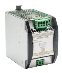
RHINO PRO PSRP series switching power supply, 24 VDC @ 20A/480W (adjustable), 120/240 VAC nominal input, 1-phase, enclosed, aluminum housing, 35mm DIN rail mount, push-in spring.
