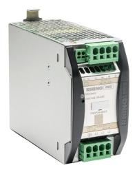
RHINO PRO PSRP series switching power supply, 24 VDC @ 20A/480W (adjustable), 480 VAC nominal input, 3-phase, enclosed, aluminum housing, 35mm DIN rail mount, push-in spring.
