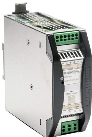
RHINO PRO PSRP series switching power supply, 24 VDC @ 5A/120W (adjustable), 120/240 VAC nominal input, 1-phase, enclosed, aluminum housing, 35mm DIN rail mount, push-in spring.
