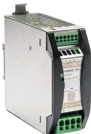
RHINO PRO PSRP series switching power supply, 24 VDC @ 5A/120W (adjustable), 480 VAC nominal input, 3-phase, enclosed, aluminum housing, 35mm DIN rail mount, push-in spring.
