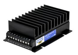
RHINO PRO DC to DC converter, 9-36 VDC input, 15 VDC output, 10A, 150W, aluminum housing, encapsulated, chassis mount, screw terminal.
