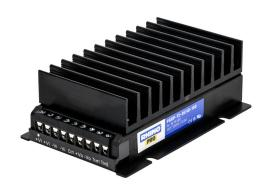
RHINO PRO DC to DC converter, 18-75 VDC input, 12 VDC output, 12.5A, 150W, aluminum housing, encapsulated, chassis mount, screw terminal.
