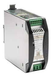
RHINO PRO PSRP series switching power supply, 12 VDC @ 10A/120W (adjustable), 120/240 VAC nominal input, 1-phase, enclosed, aluminum housing, 35mm DIN rail mount, push-in spring.
