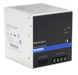
RHINO PSR series switching power supply, 24 VDC @ 40A/960W (adjustable), 480 VAC nominal input, 3-phase, enclosed, aluminum housing, 35mm DIN rail mount, screw terminals.
