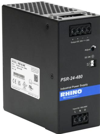
RHINO PSR series switching power supply, 24 VDC @ 20A/480W (adjustable), 120/240 VAC nominal input, 1-phase, enclosed, metal housing, 35mm DIN rail mount, screw terminals.
