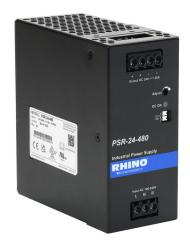
RHINO PSR series switching power supply, 24 VDC @ 20A/480W (adjustable), 120/240 VAC nominal input, 1-phase, enclosed, metal housing, 35mm DIN rail mount, screw terminals.
