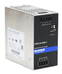
RHINO PSR series switching power supply, 24 VDC @ 20A/480W (adjustable), 480 VAC nominal input, 3-phase, enclosed, aluminum housing, 35mm DIN rail mount, screw terminals.
