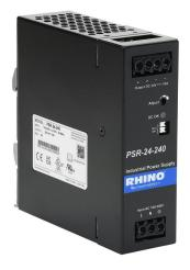
RHINO PSR series switching power supply, 24 VDC @ 10A/240W (adjustable), 120/240 VAC nominal input, 1-phase, enclosed, metal housing, 35mm DIN rail mount, screw terminals.
