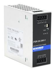
RHINO PSR series switching power supply, 24 VDC @ 10A/240W (adjustable), 480 VAC nominal input, 3-phase, enclosed, aluminum housing, 35mm DIN rail mount, screw terminals.
