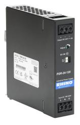
RHINO PSR series switching power supply, 24 VDC @ 5A/120W (adjustable), 120/240 VAC nominal input, 1-phase, enclosed, metal housing, 35mm DIN rail mount, screw terminals.
