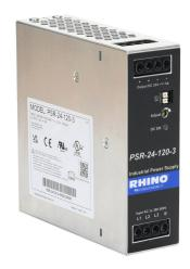
RHINO PSR series switching power supply, 24 VDC @ 5A/120W (adjustable), 480 VAC nominal input, 3-phase, enclosed, aluminum housing, 35mm DIN rail mount, screw terminals.
