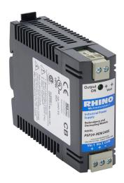
RHINO redundancy module, 2 inputs, 5/12/24 VDC nominal input, 4-59 VDC output, 8A, removable screw terminals. Requires (2) matched 24 VDC power supplies.
