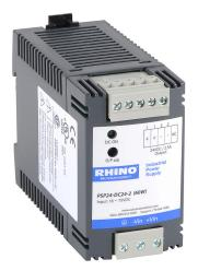
RHINO DC to DC converter, 18-75 VDC input, 24 VDC output, 2.5A, 60W, plastic housing, 35mm DIN rail mount, screw terminal, removable. DIN rail insert for panel mounting included.
