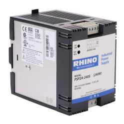
RHINO SELECT PSP series switching power supply, 24 VDC @ 10A/240W (adjustable), 120/240 VAC nominal input, 1-phase, enclosed, plastic housing, 35mm DIN rail or chassis mount, removable screw terminal.
