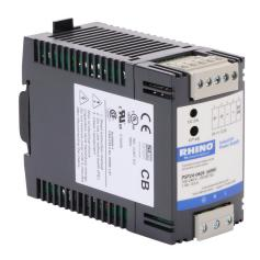
RHINO SELECT PSP series switching power supply, 24 VDC @ 2.5A/60W (adjustable), 120/240 VAC or 85-375 VDC nominal input, 1-phase, enclosed, plastic housing, 35mm DIN rail or chassis mount, removable screw terminal.
