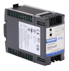
RHINO SELECT PSP series switching power supply, 24 VDC @ 2.5A/60W (adjustable), 120/240 VAC or 85-375 VDC nominal input, 1-phase, enclosed, plastic housing, 35mm DIN rail or chassis mount, spring clamp terminals.
