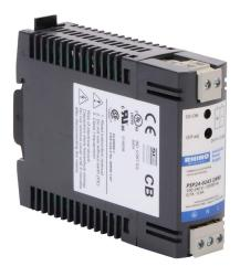
RHINO SELECT PSP series switching power supply, 24 VDC @ 1A/24W (adjustable), 120/240 VAC or 85-375 VDC nominal input, 1-phase, enclosed, plastic housing, 35mm DIN rail or chassis mount, removable screw terminal.
