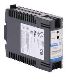
RHINO SELECT PSP series switching power supply, 24 VDC @ 1A/24W (adjustable), 120/240 VAC or 85-375 VDC nominal input, 1-phase, enclosed, plastic housing, 35mm DIN rail or chassis mount, spring clamp terminals.
