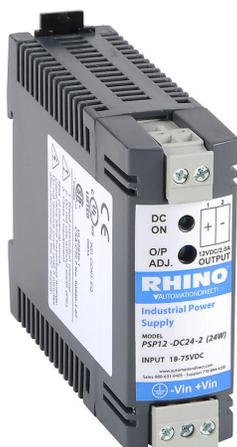
RHINO DC to DC converter, 18-75 VDC input, 12 VDC output, 2A, 25W, plastic housing, 35mm DIN rail mount, screw terminal, removable. DIN rail insert for panel mounting included.
