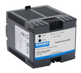
RHINO SELECT PSP series switching power supply, 12 VDC @ 8A/96W (adjustable), 120/240 VAC or 85-375 VDC nominal input, 1-phase, enclosed, plastic housing, 35mm DIN rail or chassis mount, spring clamp terminals.
