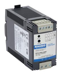
RHINO SELECT PSP series switching power supply, 12 VDC @ 4A/48W (adjustable), 120/240 VAC or 85-375 VDC nominal input, 1-phase, enclosed, plastic housing, 35mm DIN rail or chassis mount, removable screw terminal.
