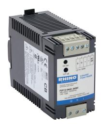
RHINO SELECT PSP series switching power supply, 12 VDC @ 4A/48W (adjustable), 120/240 VAC or 85-375 VDC nominal input, 1-phase, enclosed, plastic housing, 35mm DIN rail or chassis mount, removable screw terminal.
