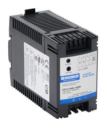
RHINO SELECT PSP series switching power supply, 12 VDC @ 4A/48W (adjustable), 120/240 VAC or 85-375 VDC nominal input, 1-phase, enclosed, plastic housing, 35mm DIN rail or chassis mount, spring clamp terminals.
