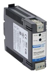
RHINO SELECT PSP series switching power supply, 12 VDC @ 2A/24W (adjustable), 120/240 VAC or 85-375 VDC nominal input, 1-phase, enclosed, plastic housing, 35mm DIN rail or chassis mount, removable screw terminal.
