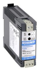
RHINO DC to DC converter, 18-75 VDC input, 5 VDC output, 5A, 25W, plastic housing, 35mm DIN rail mount, screw terminal, removable. DIN rail insert for panel mounting included.
