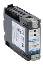
RHINO SELECT PSP series switching power supply, 5-5.25 VDC output, 4A, 20W, 120/240 VAC or 85-375 VDC nominal input, 1-phase, enclosed, plastic housing, 35mm DIN rail or chassis mount, removable screw terminal.
