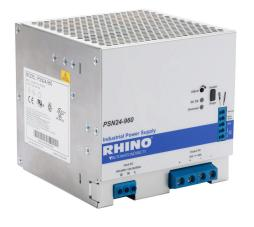
RHINO PRO PSN series switching power supply, 24 VDC @ 40A/960W (adjustable), 120/240 VAC nominal input, 1-phase, enclosed, aluminum housing, 35mm DIN rail mount, screw terminals.
